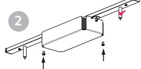
Insert power supply and attach mounting box to the track. (Mounting box can also be attached to ceiling directly using longer screws included.)
